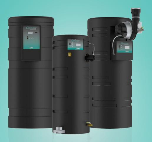
CONQUES<sup>®</sup> condensing, gas-fired water heaters are constructed from AquaPLEX® duplex stainless steel so they're corrosion-resistant in potable water at any temperature. Available in 199-1000 MBH, Conquest provides even more BTUs in small spaces and fits through a standard 36-inch doorway. With a thermal efficiency of up to 96%, long product life and a 15-year tank and heat exchanger warranty, you can't afford not to have one.
